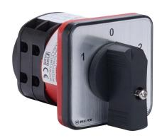
Merz rotary transfer cam switch, 2-pole, 600 VAC, 25A, 5kA SCCR, door mount, front operated. Hardware for 4-hole door mounting & black operating handle included.
