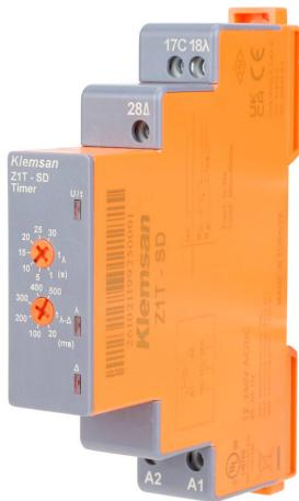
Klemsan star-delta relay timer, 1–30 seconds / 20–500 miliseconds selectable timing range, 12–240 VAC/VDC operating voltage, 10A contact rating, (1) SPDT timed relay output(s), 35mm DIN rail mount, screw terminal(s).
