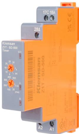
Klemsan star-delta relay timer, 1–30 seconds / 20–500 milliseconds selectable timing range, 150–500 VAC operating voltage, 10A contact rating, (1) DPDT timed relay output(s), 35mm DIN rail mount, screw terminal(s).
