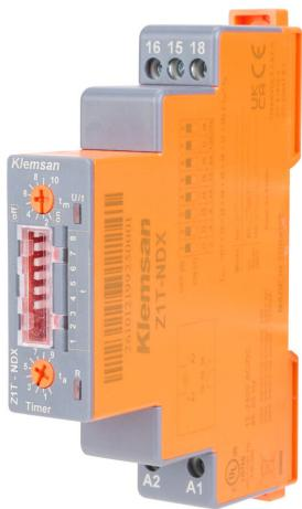
Klemsan on-delay relay timer, 0–5,109 seconds selectable timing range, 12–240 VAC/VDC operating voltage, 10A contact rating, (1) SPDT timed relay output(s), 35mm DIN rail mount, screw terminal(s).
