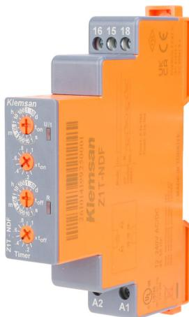
Klemsan on-flasher relay timer, 0.1 seconds to 10 days selectable timing range, 12–240 VAC/VDC operating voltage, 10A contact rating, (1) SPDT timed relay output(s), 35mm DIN rail mount, screw terminal(s).
