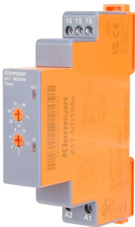
Klemsan on-delay relay timer, 1–100 seconds selectable timing range, 12–240 VAC/VDC operating voltage, 10A contact rating, (1) SPDT timed relay output(s), 35mm DIN rail mount, screw terminal(s).
