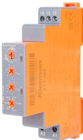
Klemsan multi-mode delay relay timer, 0.1 seconds to 10 days selectable timing range, 12–240 VAC/VDC operating voltage, 10A contact rating, (1) SPDT timed relay output(s), 35mm DIN rail mount, screw terminal(s).
