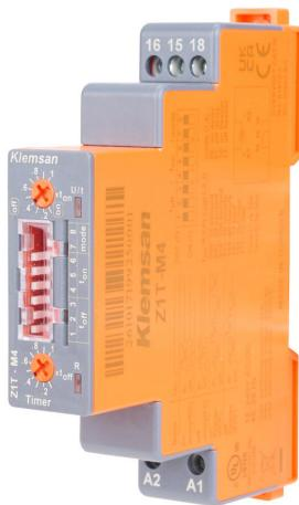
Klemsan multi-mode relay timer, 1 seconds to 10 days selectable timing range, 12–240 VAC/VDC operating voltage, 10A contact rating, (1) SPDT timed relay output(s), 35mm DIN rail mount, screw terminal(s).
