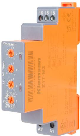
Klemsan multi-mode delay relay timer, 0.1 seconds to 99.9 hours selectable timing range, 12-240 VAC/VDC operating voltage, 10A contact rating, (1) SPDT timed relay output(s), 35mm DIN rail mount, screw terminal(s).
