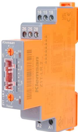
Klemsan left-right relay timer, 0.1 seconds to 10 days selectable timing range, 12–240 VAC/VDC operating voltage, 10A contact rating, (1) DPDT timed relay output(s), 35mm DIN rail mount, screw terminal(s).
