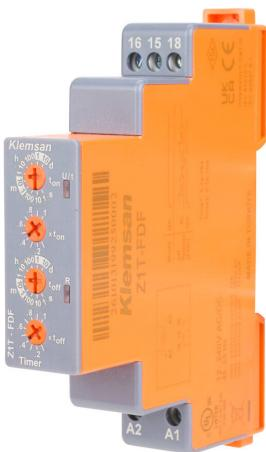
Klemsan off-flasher relay timer, 0.1 seconds to 10 days selectable timing range, 12-240 VAC/VDC operating voltage, 10A contact rating, (1) SPDT timed relay output(s), 35mm DIN rail mount, screw terminal(s).
