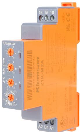
Klemsan triggered delay relay timer, 0.1 seconds to 99.9 hours selectable timing range, 12–240 VAC/VDC operating voltage, 10A contact rating, (1) SPDT timed relay output(s), 35mm DIN rail mount, screw terminal(s).
