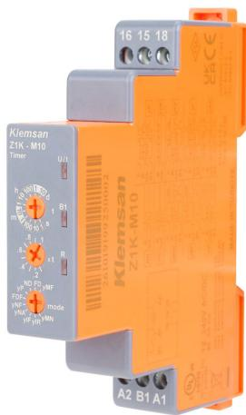
Klemsan multi-mode relay timer, 0.1 seconds to 10 days selectable timing range, 12–240 VAC/VDC operating voltage, 10A contact rating, (1) SPDT timed relay output(s), 35mm DIN rail mount, screw terminal(s).
