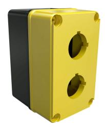
AttaBox Commander series pushbutton enclosure, 2 holes, 30mm, NEMA 1/3R/4X/6P/12, 5 x 3 x 3in (HxWxD), polycarbonate, yellow cover/black body, screw cover.
