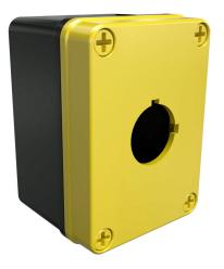
AttaBox Commander series pushbutton enclosure, 1 hole, 30mm, NEMA 1/3R/4X/6P/12, 4 x 3 x 2in (HxWxD), polycarbonate, yellow cover/black body, screw cover.
