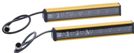
Contrinex safety light curtain, sender/receiver pair, hand protection, 24 VDC, 30mm resolution, 170mm protected height, 0.25-5.0m operating distance, safety category Type 4, configurable, IP65, (1) 5-pin and (1) 8-pin M12 quick-disconnect.
