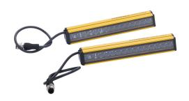
Contrinex safety light curtain, sender/receiver pair, finger protection, 24 VDC, 14mm resolution, 170mm protected height, 0.4-5.0m operating distance, safety category Type 4, configurable, IP65, (1) 5-pin and (1) 8-pin M12 quick-disconnect.
