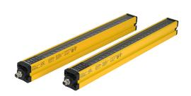
Contrinex safety light curtain, sender/receiver pair, hand protection, 24 VDC, 30mm resolution, 403mm protected height, 0.25-12m operating distance, safety category Type 4, IP65 IP67, (2) 5-pin M12 quick-disconnects.
