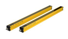
Contrinex safety light curtain, sender/receiver pair, finger protection, 24 VDC, 14mm resolution, 653mm protected height, 0.25-3.5m operating distance, safety category Type 4, IP65 IP67, (2) 5-pin M12 quick-disconnects.
