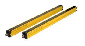
Contrinex safety light curtain, sender/receiver pair, finger protection, 24 VDC, 14mm resolution, 653mm protected height, 0.25-3.5m operating distance, safety category Type 4, IP65 IP67, (2) 5-pin M12 quick-disconnects.
