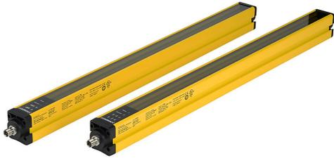
Contrinex safety light curtain, sender/receiver pair, finger protection, 24 VDC, 14mm resolution, 524mm protected height, 0.25-3.5m operating distance, safety category Type 4, IP65 IP67, (2) 5-pin M12 quick-disconnects.
