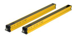
Contrinex safety light curtain, sender/receiver pair, finger protection, 24 VDC, 14mm resolution, 524mm protected height, 0.25-3.5m operating distance, safety category Type 4, IP65 IP67, (2) 5-pin M12 quick-disconnects.
