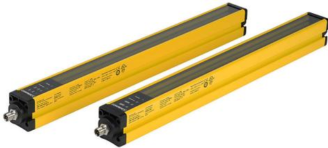
Contrinex safety light curtain, sender/receiver pair, finger protection, 24 VDC, 14mm resolution, 395mm protected height, 0.25-3.5m operating distance, safety category Type 4, IP65 IP67, (2) 5-pin M12 quick-disconnects.
