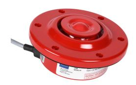
STAHL YA11 series audible alarm buzzer, hazardous location rated, 100 dB at 1m, 1 kHz tone frequency, continuous tone(s), 24 VDC, panel mount, aluminium/ABS plastic housing, red, IP66, NEMA 4X.
