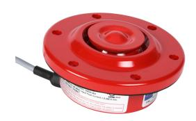
STAHL YA11 series audible alarm buzzer, hazardous location rated, 100 dB at 1m, 2.5 kHz to 3.1 kHz tone frequency, alternating fast two-tone tone(s), 24 VDC, panel mount, aluminium/ABS plastic housing, red, IP66, NEMA 4X.
