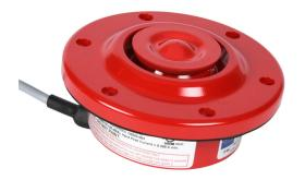
STAHL YA11 series audible alarm buzzer, hazardous location rated, 100 dB at 1m, 2.5 kHz to 3.1 kHz tone frequency, alternating fast two-tone tone(s), 24 VDC, panel mount, aluminium/ABS plastic housing, red, IP66, NEMA 4X.
