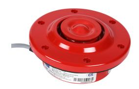
STAHL YA11 series audible alarm buzzer, hazardous location rated, 100 dB at 1m, 2.5 kHz to 3.1 kHz tone frequency, alternating two-tone tone(s), 24 VDC, panel mount, aluminium/ ABS plastic housing, red, IP66, NEMA 4X.
