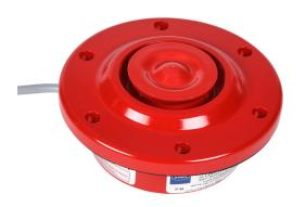
STAHL YA11 series audible alarm buzzer, hazardous location rated, 100 dB at 1m, 800 Hz to 1 kHz tone frequency, alternating two-tone tone(s), 24 VDC, panel mount, aluminium/ABS plastic housing, red, IP66, NEMA 4X.
