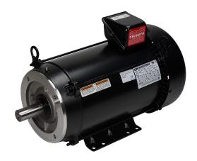
Marathon MicroMAX high efficiency AC induction motor, high-performance inverter duty, 10hp, 3-phase, 230/460 VAC, 1800rpm, TEFC, 215TC frame, rolled steel, C-face/removable rigid base mount.
