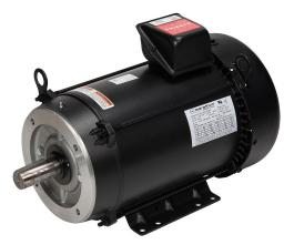
Marathon MicroMAX high efficiency AC induction motor, highperformance inverter duty, 7-1/2hp, 3-phase, 230/460 VAC, 1800rpm, TEFC, NEMA 213TC frame, rolled steel, C-face/ removable rigid base mount.
