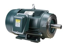
Toshiba SD premium efficiency AC induction motor, high-performance inverter duty and severe duty, 7-1/2hp, 3-phase, 230/460 VAC, 1200rpm, TEFC, NEMA 254TC frame, cast iron, C-face/rigid base mount.
