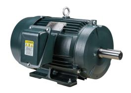
Toshiba SD premium efficiency AC induction motor, high-performance inverter duty and severe duty, 7-1/2hp, 3-phase, 230/460 VAC, 1200rpm, TEFC, NEMA 254T frame, cast iron, rigid base mount.
