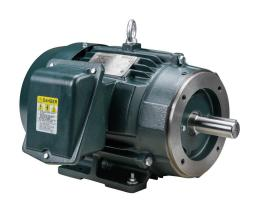
Toshiba SD premium efficiency AC induction motor, high-performance inverter duty and severe duty, 7-1/2hp, 3-phase, 230/460 VAC, 1800rpm, TEFC, NEMA 213TC frame, cast iron, C-face/rigid base mount.
