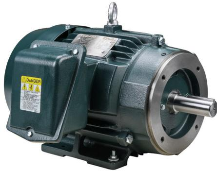
Toshiba SD premium efficiency AC induction motor, high-performance inverter duty and severe duty, 7-1/2hp, 3-phase, 230/460 VAC, 1800rpm, TEFC, NEMA 213TC frame, cast iron, C-face/rigid base mount.
