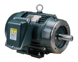
Toshiba SD premium efficiency AC induction motor, highperformance inverter duty and severe duty, 7-1/2hp, 3-phase, 230/460 VAC, 3600rpm, TEFC, NEMA 213TC frame, cast iron, Cface/rigid base mount.
