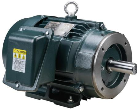
Toshiba SD premium efficiency AC induction motor, high-performance inverter duty and severe duty, 7-1/2hp, 3-phase, 230/460 VAC, 3600rpm, TEFC, NEMA 213TC frame, cast iron, C-face/rigid base mount.
