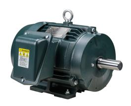
Toshiba SD premium efficiency AC induction motor, high-performance inverter duty and severe duty, 7-1/2hp, 3-phase, 230/460 VAC, 3600rpm, TEFC, NEMA 213T frame, cast iron, rigid base mount.
