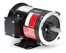
Marathon Black MAX standard efficiency AC induction motor, high-performance inverter duty, 1/4hp, 3-phase, 230/460 VAC, 1800rpm, TENV, NEMA 56C frame, rolled steel, C-face/removable rigid base mount.
