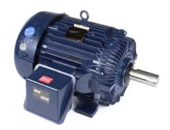
Marathon Blue MAX high efficiency AC induction motor, high-performance inverter duty, 100hp, 3-phase, 230/460 VAC, 1800rpm, TEFC, 405T frame, cast iron, rigid base mount.
