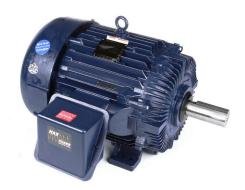
Marathon Blue MAX high efficiency AC induction motor, high-performance inverter duty, 100hp, 3-phase, 230/460 VAC, 1800rpm, TEFC, NEMA 405T frame, cast iron, rigid base mount. Dynapar HS35 encoder included.
