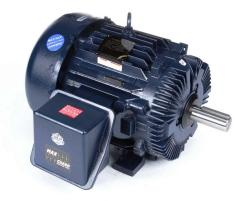
Marathon Blue MAX standard efficiency AC induction motor, highperformance inverter duty, 60hp, 3-phase, 230/460 VAC, 1800rpm, TEFC, NEMA 364T frame, cast iron, rigid base mount.
