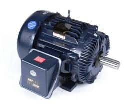
Marathon Blue MAX standard efficiency AC induction motor, high-performance inverter duty, 60hp, 3-phase, 230/460 VAC, 1800rpm, TEFC, NEMA 364T frame, cast iron, rigid base mount. Dynapar HS35 encoder included.
