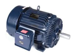
Marathon Blue MAX standard efficiency AC induction motor, high-performance inverter duty, 50hp, 3-phase, 230/460 VAC, 1800rpm, TEFC, NEMA 326T frame, cast iron, rigid base mount.
