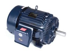
Marathon Blue MAX standard efficiency AC induction motor, high-performance inverter duty, 50hp, 3-phase, 230/460 VAC, 1800rpm, TEFC, NEMA 326T frame, cast iron, rigid base mount. Dynapar HS35 encoder included.
