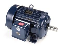
Marathon Blue MAX standard efficiency AC induction motor, high-performance inverter duty, 40hp, 3-phase, 230/460 VAC, 1800rpm, TEFC, 324T frame, cast iron, rigid base mount.
