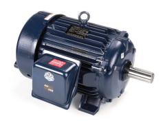
Marathon Blue MAX standard efficiency AC induction motor, high-performance inverter duty, 40hp, 3-phase, 230/460 VAC, 1800rpm, TEFC, NEMA 324T frame, cast iron, rigid base mount.
