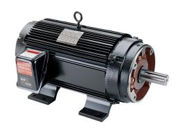
Marathon Black MAX high efficiency AC induction motor, high-performance inverter duty, 7-1/2hp, 3-phase, 575 VAC, 1800rpm, TENV, NEMA 213TC frame, cast aluminum, C-face/rigid base mount.
