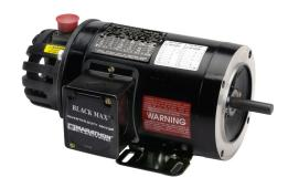
Marathon Black MAX high efficiency AC induction motor, high-performance inverter duty, 7-1/2hp, 3-phase, 575 VAC, 1800rpm, TENV, NEMA 213TC frame, cast aluminum, C-face/rigid base mount. Dynapar HS35 encoder included.
