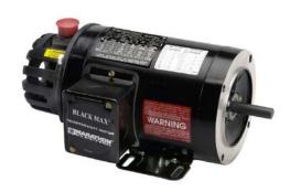
Marathon Black MAX high efficiency AC induction motor, high-performance inverter duty, 7-1/2hp, 3-phase, 575 VAC, 1800rpm, TENV, 213TC frame, cast aluminum, C-face/rigid base mount. Dynapar HS35 encoder included.
