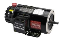
Marathon Black MAX high efficiency AC induction motor, high-performance inverter duty, 3hp, 3-phase, 575 VAC, 1800rpm, TENV, NEMA 182TC frame, aluminum, C-face/rigid base mount. Dynapar HS35 encoder included.
