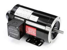
Marathon Black MAX high efficiency AC induction motor, high-performance inverter duty, 1hp, 3-phase, 575 VAC, 1800rpm, TENV, NEMA 56C frame, rolled steel, C-face/removable rigid base mount.
