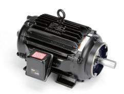
Marathon Black MAX premium efficiency AC induction motor, high-performance inverter duty, 20hp, 3-phase, 230/460 VAC, 1800rpm, TENV, NEMA 256TC frame, cast iron, C-face/rigid base mount.
