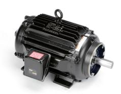
Marathon Black MAX premium efficiency AC induction motor, high-performance inverter duty, 20hp, 3-phase, 230/460 VAC, 1800rpm, TENV, 256TC frame, cast iron, C-face/rigid base mount.
