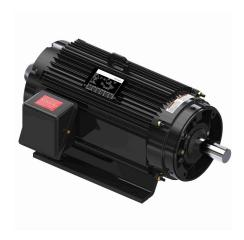
Marathon Black MAX premium efficiency AC induction motor, high-performance inverter duty, 15hp, 3-phase, 230/460 VAC, 1800rpm, TENV, NEMA 254TC frame, cast aluminum, C-face/rigid base mount.
