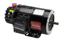
Marathon Black MAX high efficiency AC induction motor, high-performance inverter duty, 10hp, 3-phase, 230/460 VAC, 1200rpm, TENV, 256TC frame, cast aluminum, C-face/rigid base mount. Dynapar HS35 encoder included.
