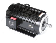
Marathon Black MAX high efficiency AC induction motor, highperformance inverter duty, 10hp, 3-phase, 230/460 VAC, 1800rpm, TENV, NEMA 215TC frame, cast aluminum, C-face/rigid base mount.
