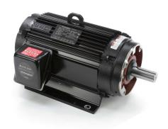
Marathon Black MAX standard efficiency AC induction motor, high-performance inverter duty, 7-1/2hp, 3-phase, 230/460 VAC, 1200rpm, TENV, NEMA 254TC frame, cast aluminum, C-face/rigid base mount.
