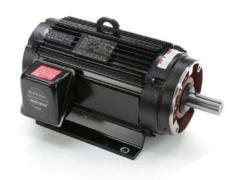
Marathon Black MAX standard efficiency AC induction motor, high-performance inverter duty, 7-1/2hp, 3-phase, 230/460 VAC, 1200rpm, TENV, 254TC frame, cast aluminum, C-face/rigid base mount.
