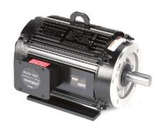
Marathon Black MAX high efficiency AC induction motor, high-performance inverter duty, 7-1/2hp, 3-phase, 230/460 VAC, 1800rpm, TENV, 213TC frame, cast aluminum, C-face/rigid base mount.
