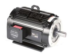
Marathon Black MAX high efficiency AC induction motor, high-performance inverter duty, 7-1/2hp, 3-phase, 230/460 VAC, 1800rpm, TENV, NEMA 213TC frame, cast aluminum, C-face/rigid base mount.
